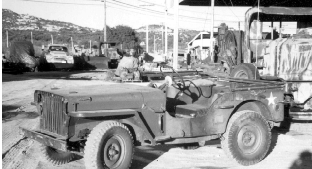
MTM's 1942 Kurtis Jeep replica, awaiting installation of its windshield, features an early WWII Ford GP-style grille.
